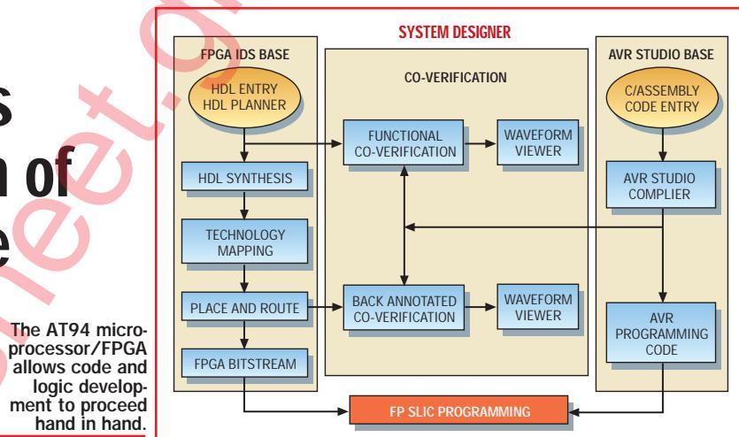
The AT94 micro-processor/FPGA allows code and logic development to proceed hand in hand.
